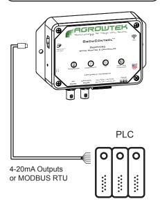
Agrowtek's sensors are easy to implement on PLC systems with 4-channel 4-20mA outputs for simple analog connections or MODBUS RTU for more advanced communication. 24Vdc is provided by the mini-din analog port or the RJ45 MODBUS port for single-cable installation.
