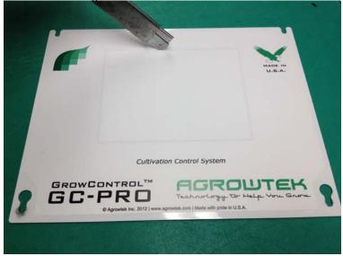
4. Place the panel on a block of wood and use a chisel punch and hammer to break the knock-out tabs. Remove the knock-out panel. Be careful not to bend the front panel in the process.
