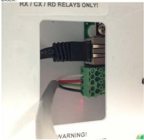
11. Install the touch screen's power cable (red/black/blue wires) to the "HMI" power port on the power bus circuit board.
