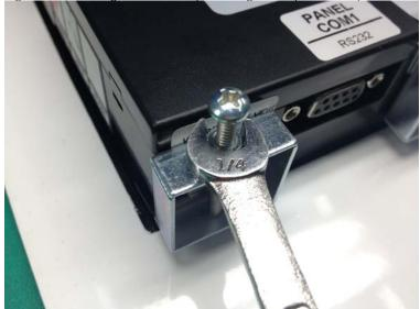
Install the data cable to the bottom of the touch panel securing with two screws provided.
