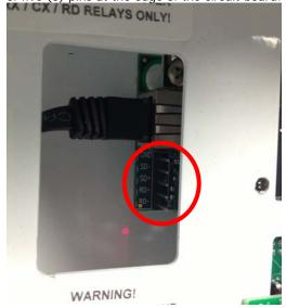
10. Install the data cable's green terminal block onto the pin header, ensuring the five pins are all properly aligned and then press backwards. A small screw driver or needle-nose pliers will assist in pushing down squarely on the terminal block.
