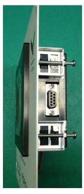
14. To complete the installation, slide the front cover back into position and tighten the four panel screws.
