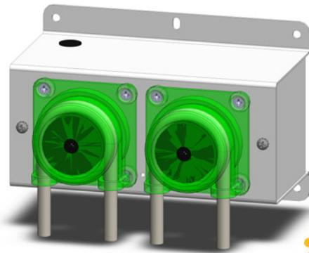
Pumps can draw solutions up to 100ft with a 10ft vertical lift and do not require priming. Peristaltic action resists fouling or clogging even with thick fluids. Durable pumps reliably deliver accurate doses. Economical quick change roller head can be replaced by rotating 1/8 turn and pulling off of motor shaft. FDA Compliant tubing and lifetime lubricant.
