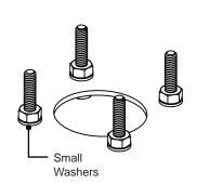
Install stainless steel bolt kit in tank. These bolts remain installed in the tank permanently. Locate the seal over the bolts.
