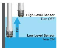
Agrowtek's automatic fill or drain control systems use two SXL level sensors to control water level reliably and precisely between two points. Systems are available with a water valve or outlet relay kit and the LSM mounting kit for a complete solution.
