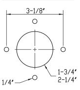
On the top of the tank, mark and drill the center hole using a hole saw, then align template or flange to mark and drill at least two bolt holes.
