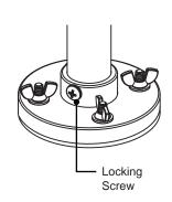
Adjust the sensor height as required and secure the locking screw. The sensor may be extracted for maintenance by removing the wing nuts.
