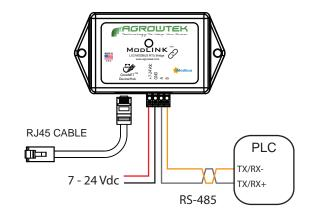
3.3/5Vdc Serial Bus Compatible. Include required bus terminating resistors per EIA standard.
