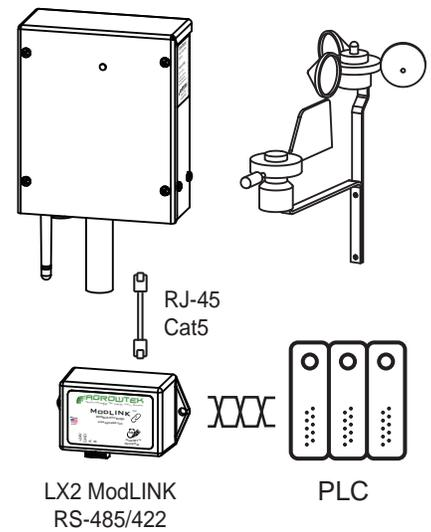
Agrowtek's sensors are easy to implement on PLC systems with MODBUS RTU and a LX2 ModLINK interface. Multiple GrowNET devices can be connected to an interface with HX8 GrowNET hubs. Sensors are also available with 4-channel 4-20mA outputs.
