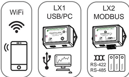
Connect the sensor directly to a computer using the LX1 USB AgrowLINK and free PC software for data logging and email alerts, or use a ModLINK LX2 RS-485 or LX4 RS-422 interface for MODBUS protocol. HX8 hubs allow multiple devices on LX interfaces. Add WiFi to monitor the sensor directly from a web browser, or link the sensor to your Agrowtek web portal account.
