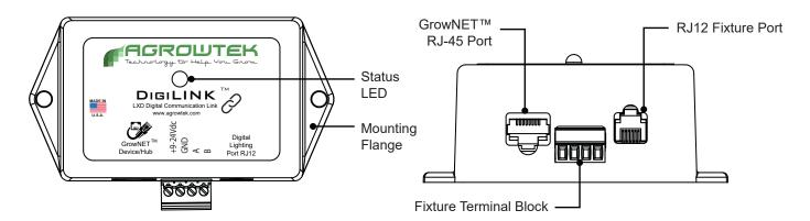
Fixtures connect to either the RJ-12 connection (see compatible fixtures above) or via manual connection to the terminal block. See wiring diagrams for connection details. A status LED will flash when communicating with the GCX controller.
