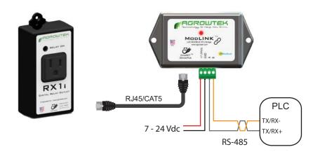
3.3/5Vdc Serial Bus Compatible. Include required bus terminating resistors per EIA standard.
