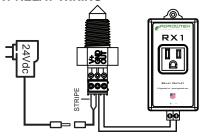
Agrowtek's RX1 is a CSA Listed 120Vac/12A relay outlet. The RX1 plugs into a wall outlet and can be wired directly to the SXL-1 or SXL-2 sensor to control any 120V device. A fly-back diode is built into the RX1 relay.
